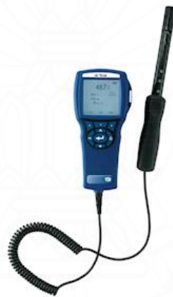
Figure 3.1 Q-Trak ® model 7575 with Model 982 IAQ Probe.
